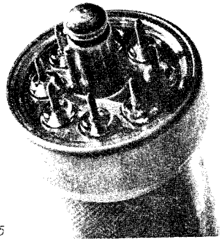
Fig. 5 The base of a key valve, showing the cut-outs for the elevations of the glass base, thereby giving a sufficiently long leakage path between the pins and the screen plate.
